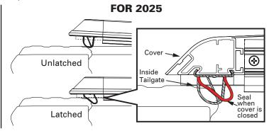
**9 REAR CLAMP OPERATION.** The rear (tail) clamps are stowed in the cover rail. Rotate the clamp down and slide it to the truck bed rail. The clamps should be slid, at a slight angle, as far over to the rail as possible. Pull the clamps straight down and release them to hook under the bottom of the metal bracket. Always latch the clamps on both sides of the bed.
