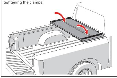
Ensure that the clamp is positioned under the previouly installed bracket. Hand tighten until clamp contacts the bracket, then tighten an additional two turns. DO NOT secure to only the lip of the bedliner or the plastic bed cap. DO NOT use a wrench or overtighten!
