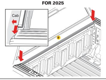
INSTALLING COVER. Note: Take care not to damage or deform the seals when installing the bed cover onto the truck bed. Visually check to ensure the front bed cover frame is even on both sides and square with the bed. Place the bed cover over the cab end and of the truck bed. Make sure the cover is centered on the bed of the vehicle before
