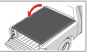
**PROPER POSITION OF TONNEAU COVER.** Close the tailgate and unfold the cover. Check that the cover is parallel and square with the truck bed and bed rails. Adjust the cover until the bulb seal fits with the tailgate as shown. If not parallel or square, open the cover and loosen the cab clamps to reposition the cover.
