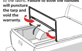
Securing the cover. To drive with the cover open, fold the cover forward to the cab and fasten BOTH straps in the middle section to the front rail. Check that the straps are tight, and pull the strap
